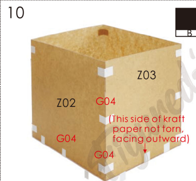
Use G04 to secure the acrylic joint (or substitute with transparent tape).
